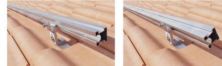
The hammer-head screw is now engaged in the mounting profile. Tighten the lock nut onto the hammer-head screw of the outermost roof hook, so that the profile can no longer rotate or slip free from the roof hook.
